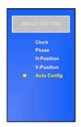
> V-Position : Adjust vertical position of the screen
